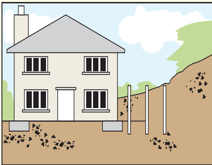
Fig. 3 100mm dia. steel tubular piles.
